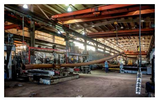
Bending steel, John L. Lutz Welding & Fabrication, Frenchtown, New Jersey, 2012
